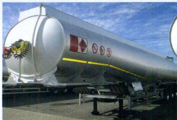
ALUMINIUM 50000L TRIDEM BRIDGING SEMITRAILER The demand for fuel tankers into Africa is increasing
